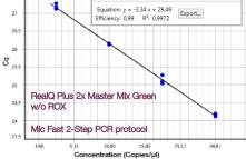
The qPCR standard curve showed a strong linear correlation between the  $C_{\rm q}$  values and log [template DNA]. The efficiency calculated from the curve slope is 99%.
