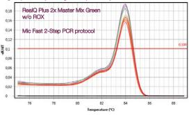
Melt curve analysis for the amplified pAH12 target. Mic software was used
